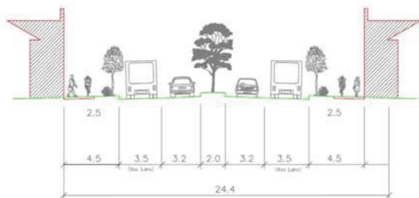
Figure 54: Wellington Road Proposed Cross-section (Walter Road West to Morley Drive)
