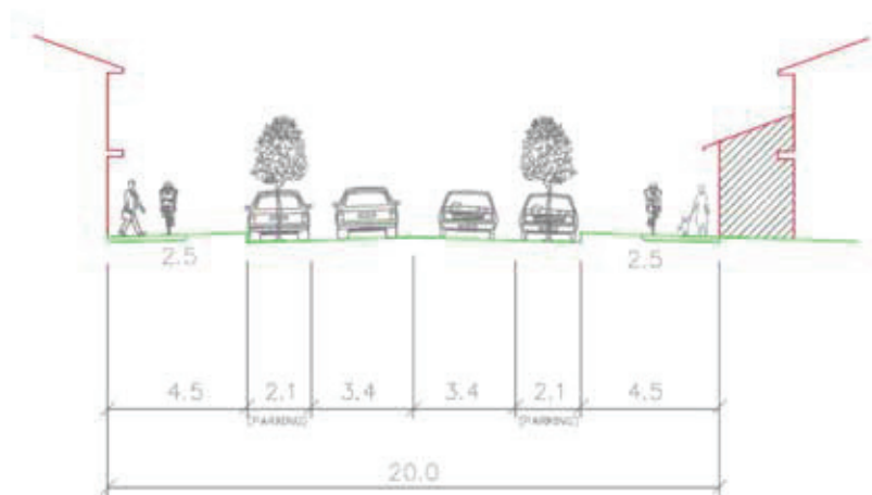
Figure 51: Drake Street Proposed Cross-section (Broun Avenue to Smith Street)
