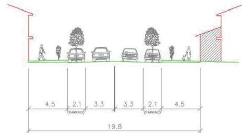
Figure 50: Rudloc Road Proposed Cross-section (Russell Street to Coode Street)
