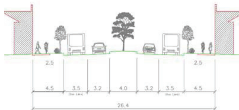
Figure 52: Walter Road West Proposed Cross-section (Wellington Road to Russell Street)
