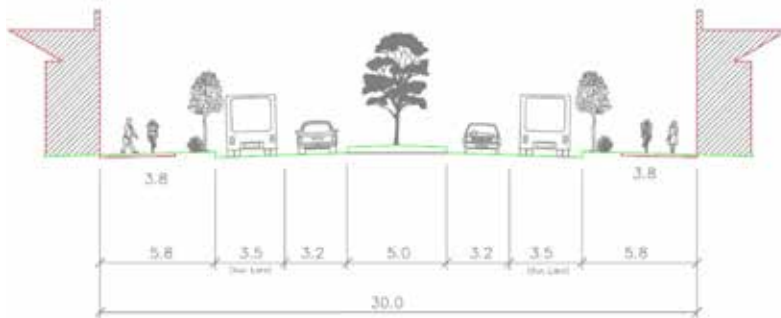
Figure 46: Broun Avenue Proposed Cross-section (Coode Street to Russell Street)
