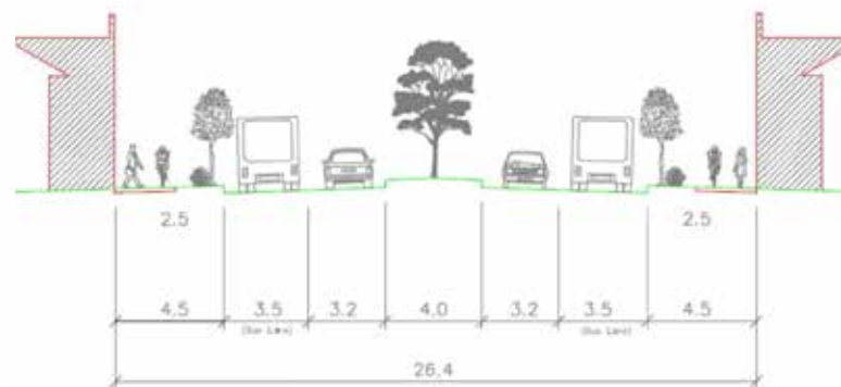
Figure 52: Walter Road West Proposed Cross-section (Wellington Road to Russell Street)
