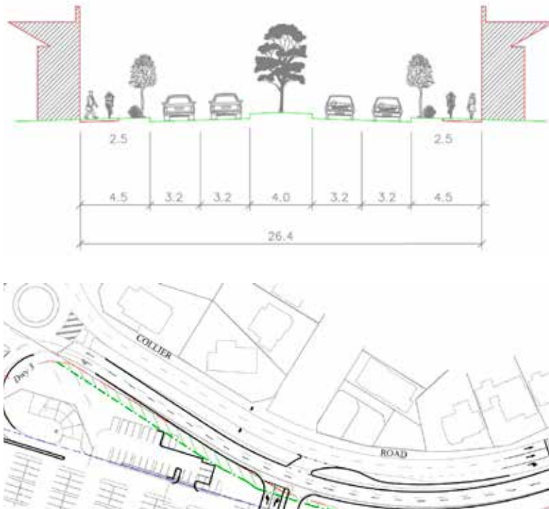
Figure 49: Collier Road Proposed Cross-section (Broun Avenue to Walter Road West)
