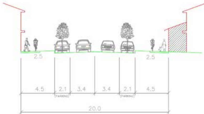
Figure 51: Drake Street Proposed Cross-section (Broun Avenue to Smith Street)
